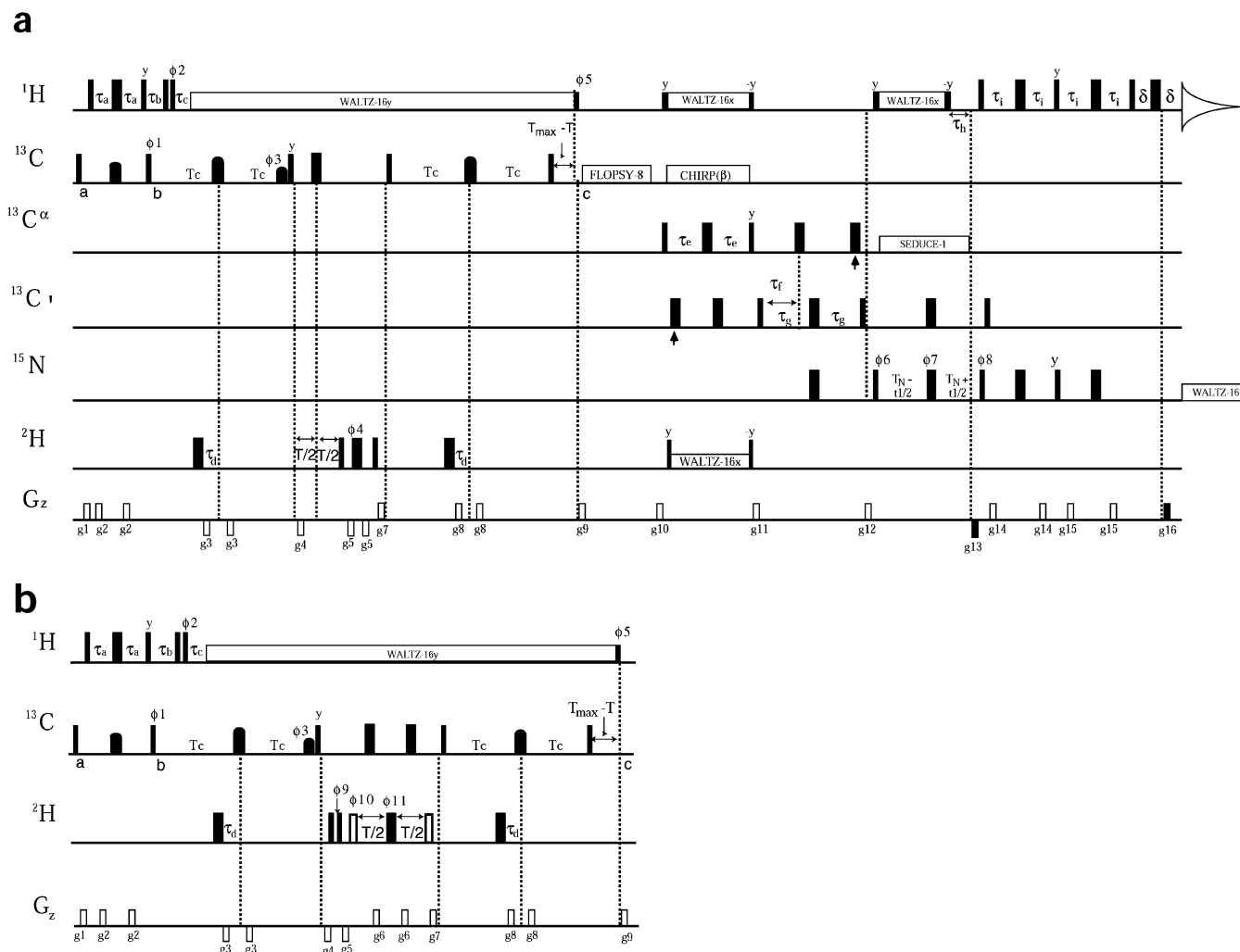
Figure 1. Pulse schemes used for the measurement of relaxation rates of deuterium quadrupolar order, 3D_Z^2 - 2, R_{3D_Z^2-2} (a), and antiphase transverse magnetization, D_+D_Z + D_ZD_+, R_{D_+D_Z+D_ZD_+} (b), in unfolded protein states. Similar pulse schemes for the measurement of R_{D_Z} and R_{D_+} in unfolded proteins have been described previously 19 (minor modifications that have recently been incorporated are available from the authors upon request). All narrow (wide) rectangular pulses correspond to flip angles of 90^\circ ( 180^\circ ) and are applied along the x -axis, unless otherwise indicated. Carriers are positioned at the water frequency ( ^1\text{H} ), 119 ppm ( ^{15}\text{N} ), 0.8 ppm ( ^2\text{H} , start of sequence until the end of the FLOPSY mixing scheme), 4.7 ppm ( ^2\text{H} , immediately after FLOPSY mixing until the end of the sequence), 20 ppm ( ^{13}\text{C} , start of sequence until FLOPSY-8), 43 ppm ( ^{13}\text{C} FLOPSY mixing), and 58 ppm ( ^{13}\text{C} , immediately after the FLOPSY-8 until the end of the sequence). All proton pulses are applied with a 32.5 kHz field, with the exception of the 6.4 kHz field used for WALTZ decoupling 66 and the pulses immediately flanking the decoupling elements (also 6.4 kHz). The ^{13}\text{C} shaped 180^\circ pulses between points a and b (1.36 ms at 600 MHz, centered at 19.5 ppm) and in the middle of the 2T_c periods (392 \mu\text{s} , 41 ppm) have RE-BURP profiles. 67 The ^{13}\text{C} pulse of phase \phi_3 (640 \mu\text{s} , centered at 57 ppm) is applied with the SEDUCE-1 shape. 68 Magnetization relay through TOCSY mixing is achieved using the FLOPSY-8 scheme (8 kHz field, 7 cycles). ^{13}\text{C}_\beta decoupling fields, centered at both 29.5 ppm ( \pm 14.5 ppm) and 70.0 ppm ( \pm 2 ppm) and denoted by CHIRP( \beta ), were implemented using a scheme comprised of 5 ms WURST-2 pulses. 69 The decoupling element was created using the Varian tool Pbox. All ^{13}\text{C}_\alpha rectangular pulses have durations which minimize excitation in the carbonyl region of the carbon spectrum and vice-versa. 70 Pulses indicated with vertical arrows are used to compensate for Bloch–Siegert effects. 71 ^{13}\text{C}_\alpha WALTZ decoupling during the constant time 2T_N period was achieved with 326 \mu\text{s} SEDUCE-1 pulses centered at 58 ppm. All ^{15}\text{N} pulses are applied with a 5.8 kHz field, with 1.1 kHz WALTZ-16 decoupling during acquisition. ^2\text{H} WALTZ decoupling employed a 0.7 kHz field; all other ^2\text{H} pulses are 2.0 kHz. The narrow rectangular pulses that are not filled in part b have flip angles of 45^\circ . The delays employed are as follows: \tau_a = 1.7 ms, \tau_b = 3.85 ms, \tau_c = 1.93 ms, T_c = 14.5 ms, \tau_d = 1.7 ms, \tau_e = 4 ms, \tau_f = 4.4 ms, \tau_g = 13.0 ms, \tau_h = 5.5 ms, \tau_i = 2.4 ms, T_N = 15 ms, and \delta = 0.5 ms. T_{\text{max}} is chosen equal to the maximum value of T (relaxation delay) that is used in the relaxation series. The phase cycling is as follows: \phi_1 = 2(x), 2(-x) ; \phi_2 = x, -x ; \phi_3 = 4(x), 4(-x) ; \phi_4 = 4(0^\circ), 4(45^\circ), 4(90^\circ), 4(135^\circ) ; \phi_5 = -x, x ; \phi_6 = 16(x), 16(-x) ; \phi_7 = 2(x), 2(-x) ; \phi_8 = x, 4(-x) ; \phi_9 = 4(x), 4(-x) ; \phi_{10} = 8(x), 8(-x) ; \phi_{11} = 16(x), 16(-x) . For part a, rec. = x, 2(-x), x, -x, 2(x), -x, x, 2(-x), x, -x, 2(x), -x . After 16 scans, the phase of the receiver is inverted. For part b, rec. = x, 2(-x), 2(x), 2(-x), x, -x, 2(x), 2(-x), 2(x), -x . After 16 scans, the phase of the receiver is inverted. The durations and strengths of the gradients are g_1 = (0.5 ms, 5 G/cm), g_2 = (0.3 ms, 3 G/cm), g_3 = (0.3 ms, -25 G/cm), g_4 = (0.2 ms, -10 G/cm), g_5 = (0.4 ms, -10 G/cm), g_6 = (0.05 ms, 25 G/cm), g_7 = (0.25 ms, 6 G/cm), g_8 = (0.2 ms, 10 G/cm), g_9 = (0.6 ms, 15 G/cm), g_{10} = (1.0 ms, 15 G/cm), g_{11} = (0.4 ms, 6 G/cm), g_{12} = (0.5 ms, 25 G/cm), g_{13} = (1.25 ms, -30 G/cm), g_{14} = (0.2 ms, 2.5 G/cm), g_{15} = (0.3 ms, 2.0 G/cm), and g_{16} = (0.125 ms, 29.6 G/cm). Quadrature detection is achieved in t_1 using the enhanced sensitivity gradient approach, 72,73 with separate FIDs recorded for each t_1 point corresponding to ( \phi_8 = x, g_{13} ) and ( \phi_8 = -x, -g_{13} ). Decoupling is interrupted prior to the application of gradients. 74
